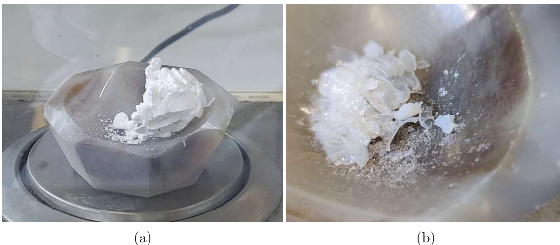
Figure 5: Pictures of 2:1 Mg:Al HT that was prepared using the (a) standard method (b) fast method.
