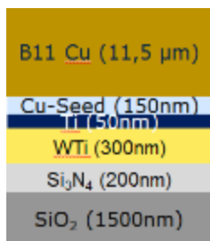
Figure 43: Sequence of layers in Wafer 7
