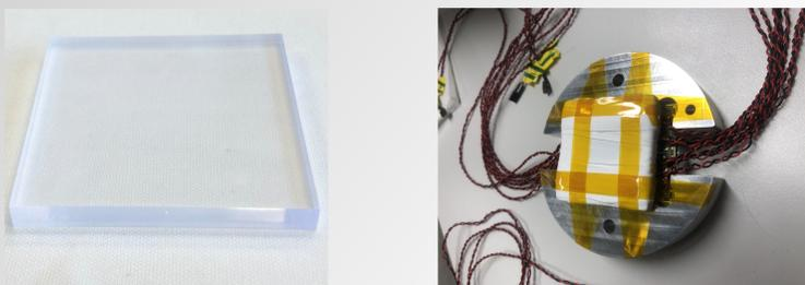
The 50 x 50 x 5 mm<sup>3</sup> plastic scintillator was wrapped in teflon tape to increase the light collection of the SiPM, which has been optically coupled to the scintillator with a silicone wafer. The aluminium holder keeps the center of the SiPM aligned with the electron beam.
