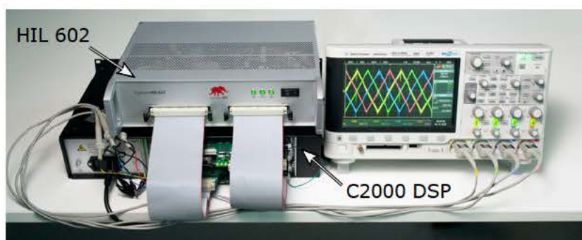
Figure 3.7: The C-HIL test setup with a TYPHOON HIL 602 and a Texas Instruments C2000 DSP.
