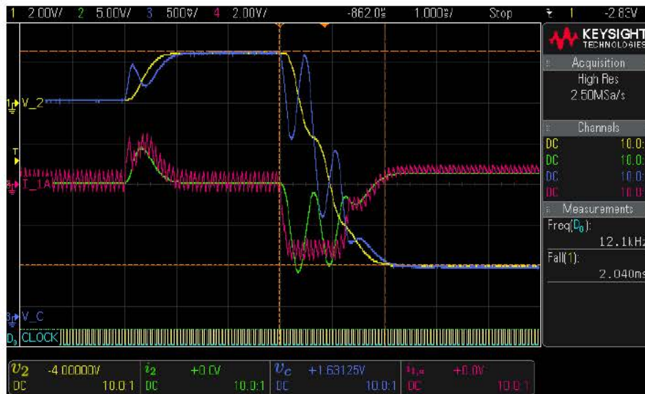
Figure 3.8: Proposed control concept on the C-HIL test bed with a switching frequency f_{\text{PWM}} = T_s^{-1} = 12 \text{ kHz} . Channel 1, 2, 3, shows the voltage v_2 , the current i_2 , and the voltage v_c respectively. Representative for all leg currents, the current i_{1,a} is shown on channel 4.
