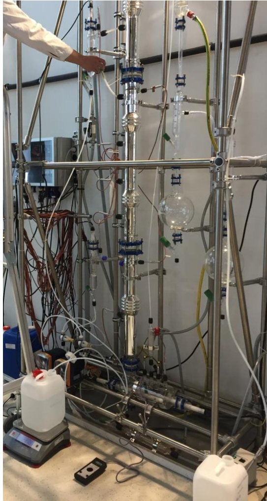
Figure 29: Setup of the pulse experiments for RTD measurements
