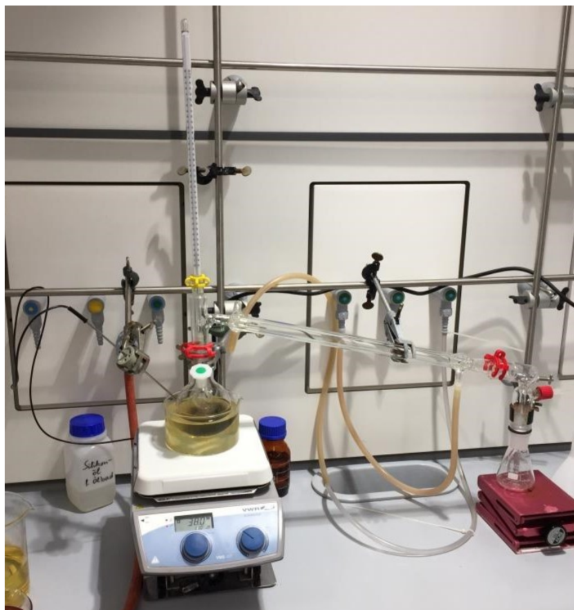
Figure 37: Experimental setup for reactive distillation in lab scale
