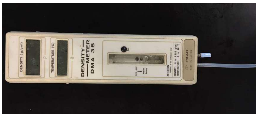
Figure 26: Handheld oscillating u-tube density meter (DMA 35 from Anton Paar GmbH)
