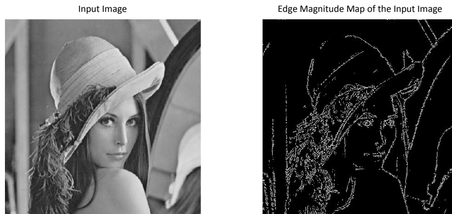
Figure 20: Transformation from Input Image to Edge Image through the Canny Edge Detector [22].
