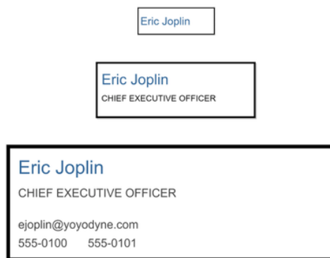
Figure 2.1: Semantic zooming in yFiles. The same object is represented in three different levels of detail. They are rendered depending on the current zoom level.
