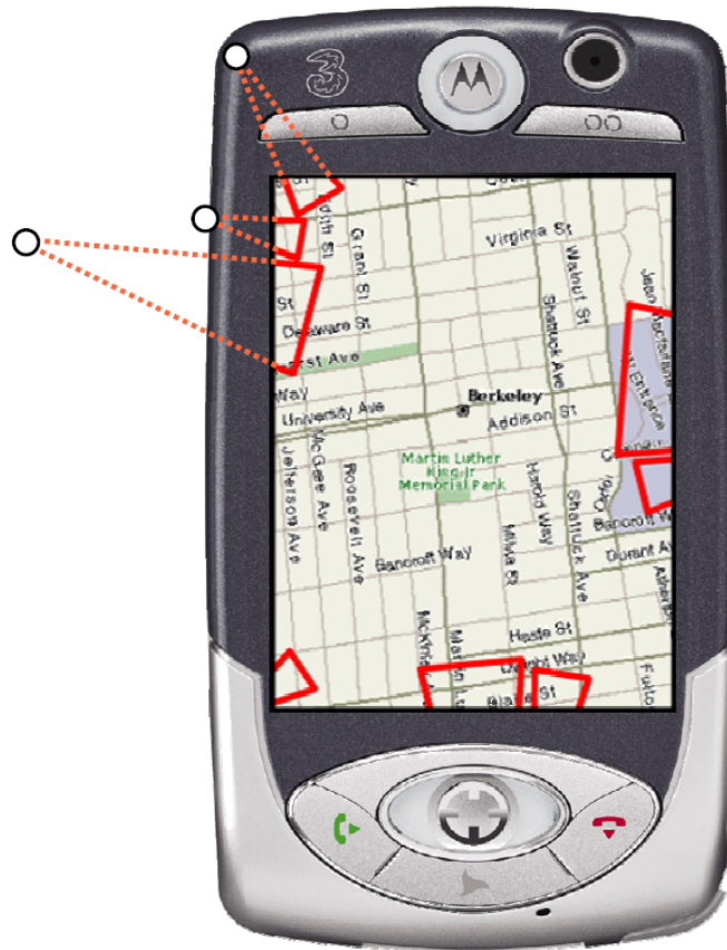
Figure 3.23: Example for wedges. A visualization technique by Gustafson et al. [GBGI08] for off-screen element visualization. Red triangles indicate existence of off-screen elements. Visible legs of triangles give information about distance. Image source: [GBGI08]
