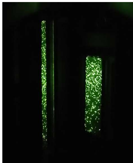
Figure 19: Real-color photo of the MCP signal of a vacuum gauge as seen through the viewport, taken with a smartphone camera. The left strip visible on the image is the actual MCP whereas the right strip is the image reflected by the mirror.
