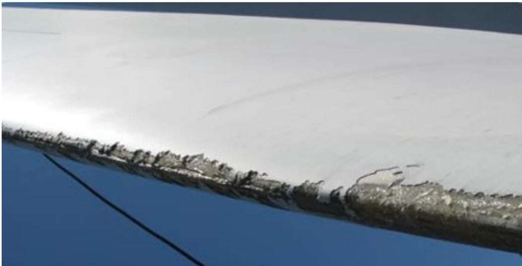
Figure 1.1: A severely eroded leading edge [3].
