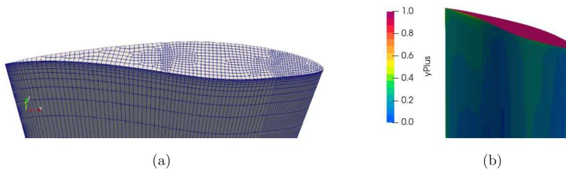
Figure 6.3: a) Surface mesh and b) contour of  $y^+$  in the blade tip region.
