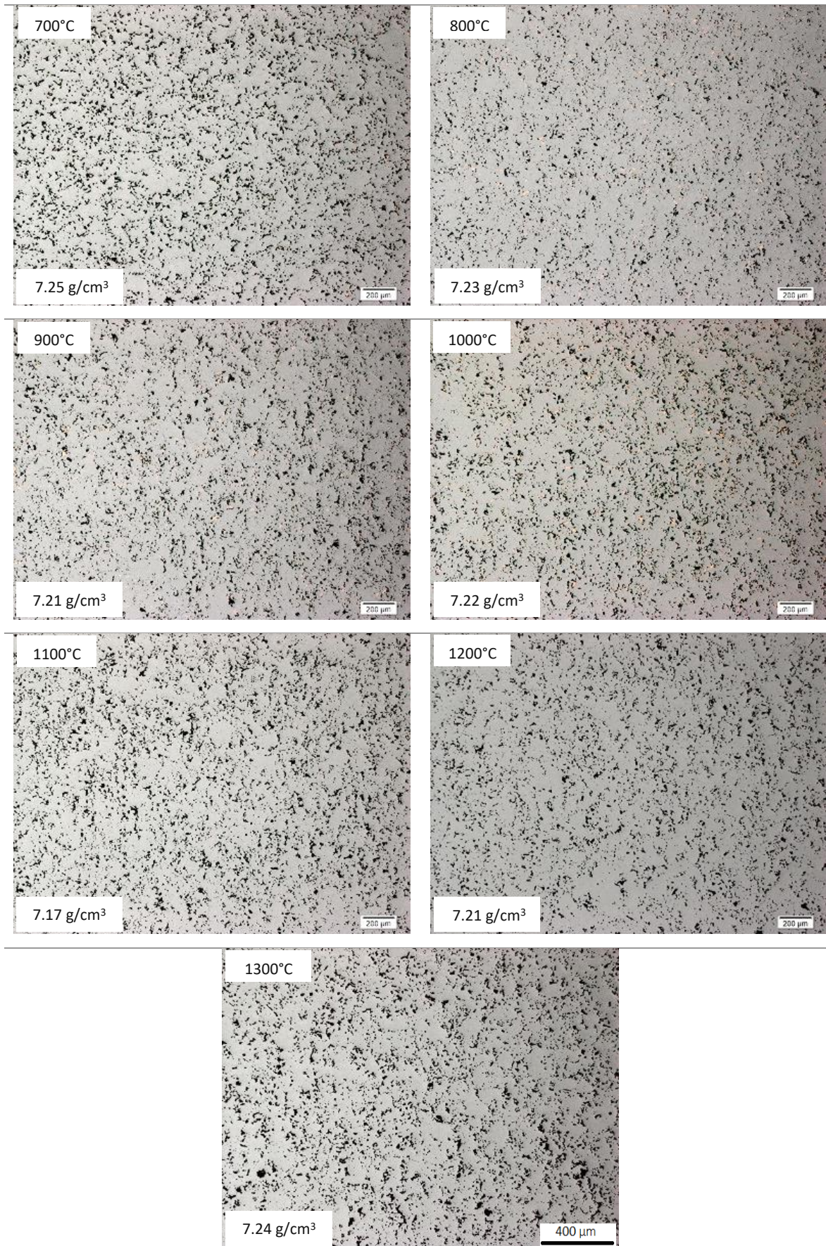
Figure 3.93: Un-etched OM micrographs of copper alloyed steel (Fe-2Cu-0.8C admixed ) compacted at 600 MPa, sintered 60 min in argon, 50 x. (scale bar 400μm holds for all images)
