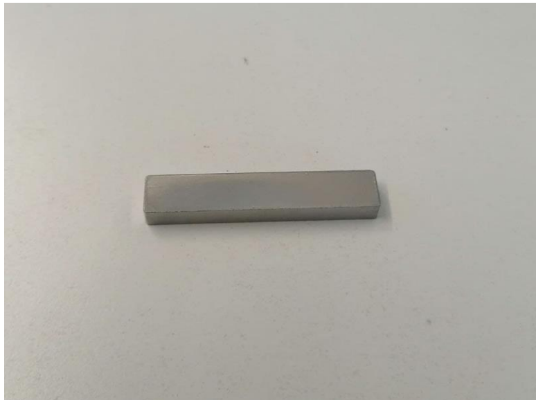
Figure 2.11: Charpy impact bar prepared for this research
