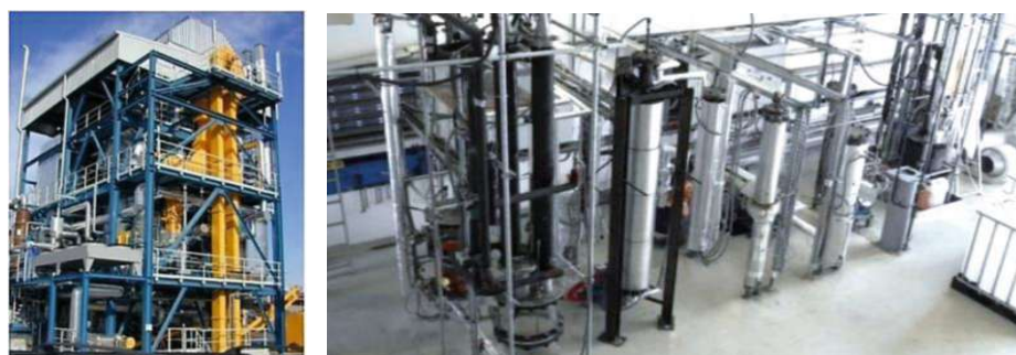
Figure 24: Combined heat and power plant Güssing (left) and laboratory-scale Fischer–Tropsch plant (right) 4
