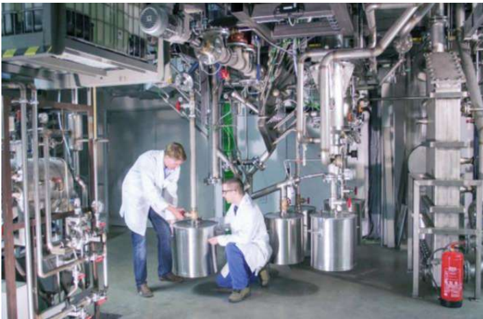
Figure 19: Gasification test plant used for the experimental validation of fuel flexible gasification 3
