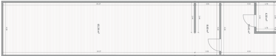
Figure 4.12: Floor plan of the studio. The outer measurements are 21.96 m \times 4.44 m and the living area is exactly 93.5 m 2 .
