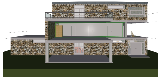
Figure 5.14: When a room is selected in the side view, all other rooms of the floor may be exploded and, therefore, be translated to a position behind the camera. They just follow their exploded major boundary walls.
