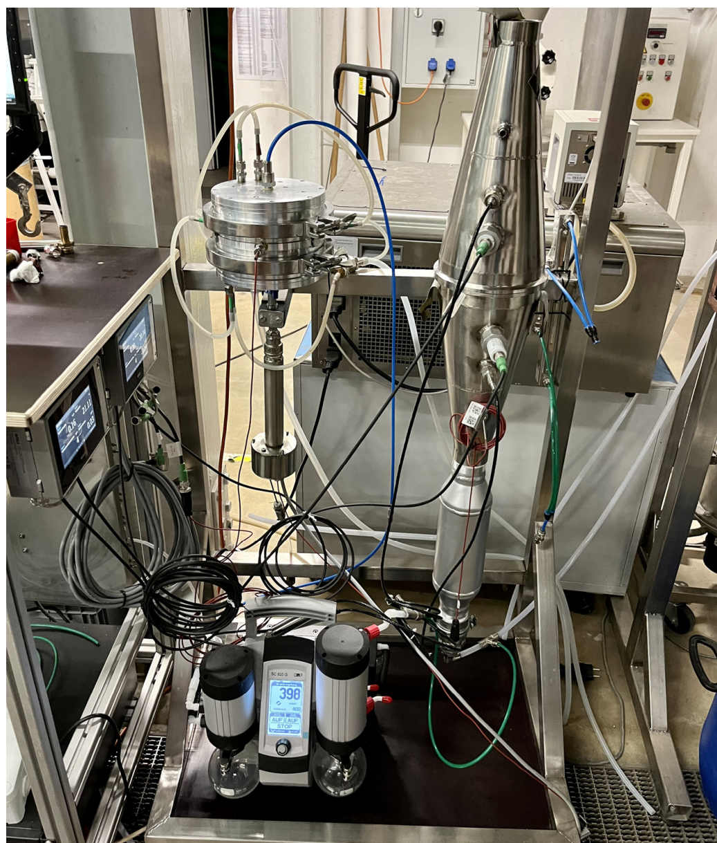
Figure 1. Experimental DAC plant set up in the Technikum at TU Wien. The system is shown in the desorption mode. In the lower part of the picture, the vacuum pump is operating at 398 mbar.
