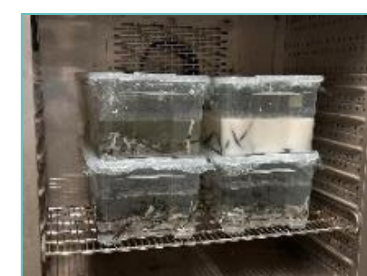
Basalt yarns in solutions heated at 60° C
