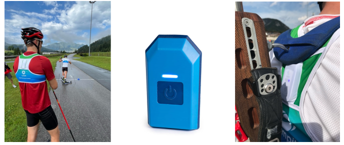
Fig. 18: OCULUS tracking device mounted on biathlon athlete.
