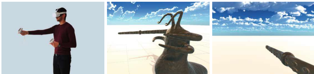
(c) Large extension of the real arm: non-linear part of the mapping function. Arm stretches accordingly.
