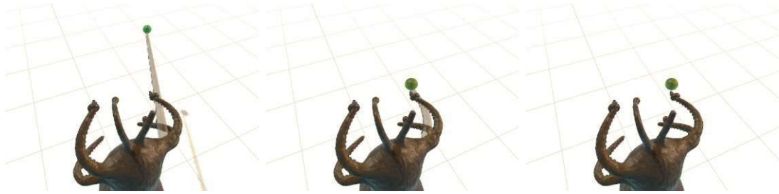
Figure 3.8: Animation of the arm halo retrieving the distant object. Once the object is close enough, the halo mesh is turned off.
