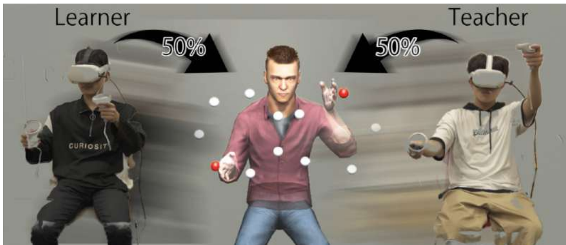
Figure 2.6: Virtual avatar controlled based on the weighted average of the teacher’s and learner’s movements in a co-embodiment scenario. [29].
