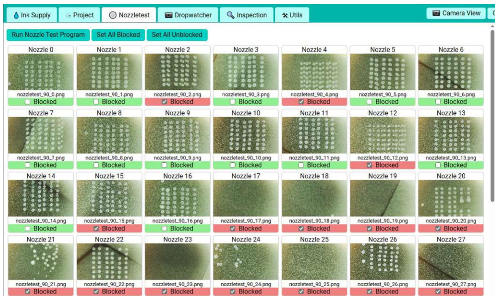
Figure 3.9: Nozzle test screen of the software: A small calibration grid is printed using each nozzle as shown. The user can select which nozzles should be used to continue the print. Nozzle 2, 4, 7, and 12 show satellite drops, 17-19, 23, 25, and 27 are blocked completely, 21 and 24 are misfiring heavily, and 15, 20, 22, and 26 show missing jets.
