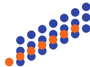
Figure 2.22: Drop overlap in print (y) direction, indicated by blue and orange dots, is generated by moving the track in move (x) direction for subsequent layers.
