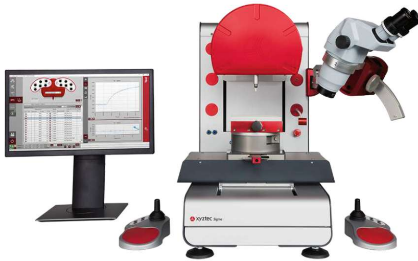
Figure 3.24: XYZ-TEC Condor Sigma device - bond tester. Copied from: https://www.xyztec.com/wp-content/uploads/2023/05/Sigma-lite-2022.png
