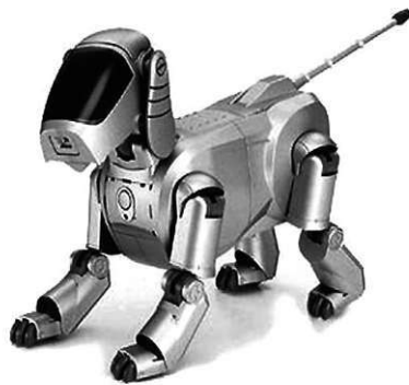
Figure 2.1: AIBO original model ERS-110, example for a socially interactive robot. Reprinted from [20]
