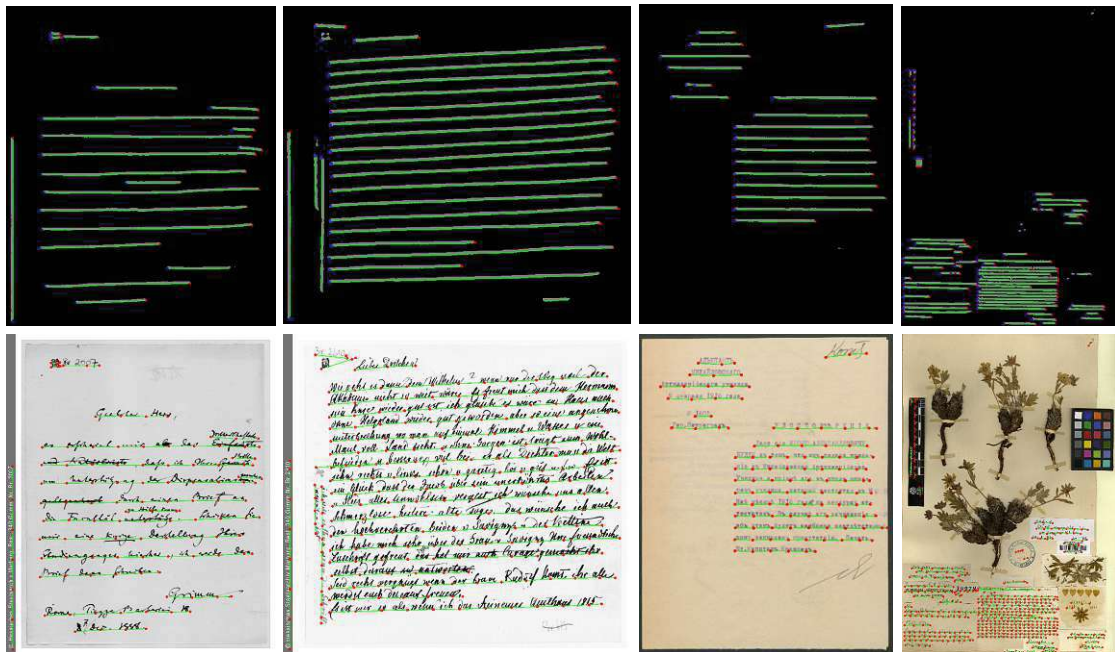
Figure 3.5: Illustrative results of the segmentation model applied to cBAD 2019 dataset test images. The first row visualizes the segmentation model’s output: initiation points (blue), termination points (red), boundary class (purple), and baselines (green) with text regions (grey). The second row presents the input image overlaid with the predicted baselines, where red dots represent the predicted baseline coordinates, connected by lines (green).
