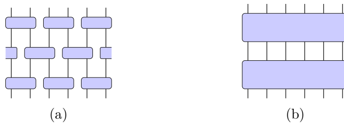
Figure 2.1: (a) Example of a spatially local quantum circuit, such an architecture is also referred to as a “brickwork” circuit in the literature. Each leg corresponds to an individual qudit while blue rectangles depict unitary gate that act on the Hilbert space of the incoming legs. By thinking of this structure in terms of a Trotterized many-body system, one can interpret it as universal approximation of a system with nearest-neighbor interactions [20]. (b) All-to-all interacting unitary circuit. In the past, this model has found many interesting applications, an example being the study of scrambling in black holes if the individual gates are sampled from the unitary Haar measure [21, 22].
