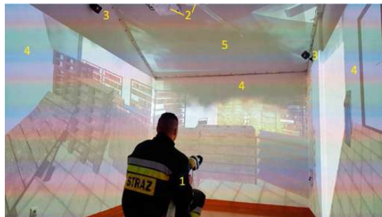
Figure 2.4: CAVE Setup for training scenario by Grabowski [28].
