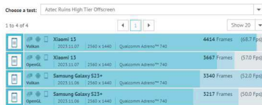
(a) 740 GPU scores of other devices between 3217 and 4414 for OpenGL and Vulkan on GFXBench
