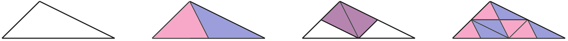
Figure 2.2: Refinement by NVB leads only to 4 similarity classes of triangles. We can see this by iterating NVB until no more new classes of triangles appear.
