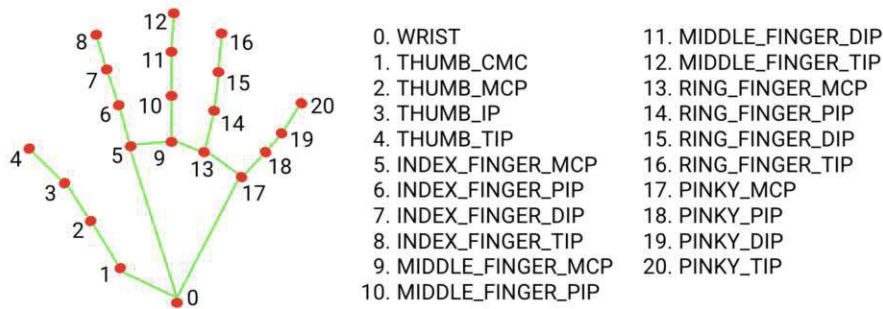
Figure 5.3: Landmark indices of the MediaPipe framework. Marked landmarks are used for hand length calculations.
