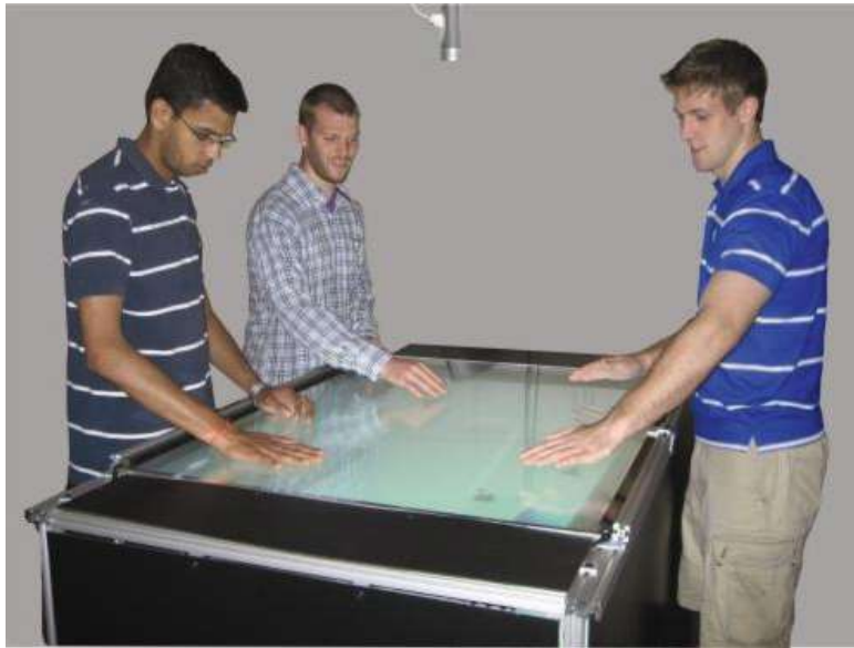
Figure 2.7: Three users interacting with the multi-touch tabletop by Dohse et al. On top is a camera attached that is used for hand tracking [18]. The image is taken the authors' work.
