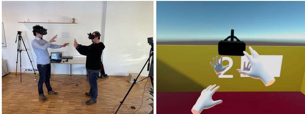
Figure 2.6: Two collocated users in both the physical and virtual space, with hand tracking enabled. The point of view (POV) is from the left user within the virtual scene.
