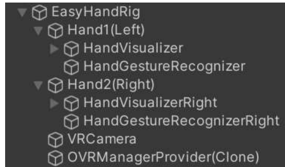
Figure 3.12: The 'EasyHandRig' inside the Unity engine. The 'EasyHandManger' component is placed on the parent 'EasyHandRig' game object. Each hand object has its own visualizer and gesture recognizer. The VR camera represents the user's HMD and is responsible for user positioning and rendering. In this example, Meta Quest hand tracking is used, which is why an OVRManager is created at runtime to obtain the low-level data of the tracking system for unification.
