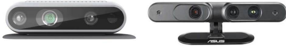
Figure 2.3: Two RGB-D cameras are depicted. Left: Intel RealSense Depth Camera D435; Right: ASUS Xtion PRO LIVE
