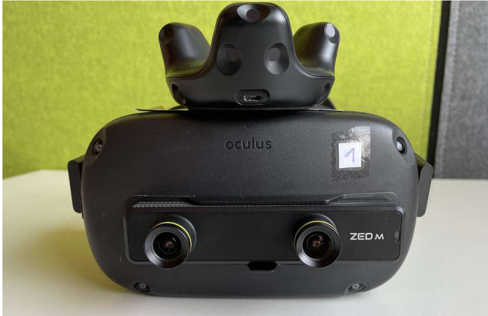
Figure 4.5: Meta Quest with an attached Vive Tracker and ZED-Mini camera used in the evaluation.
