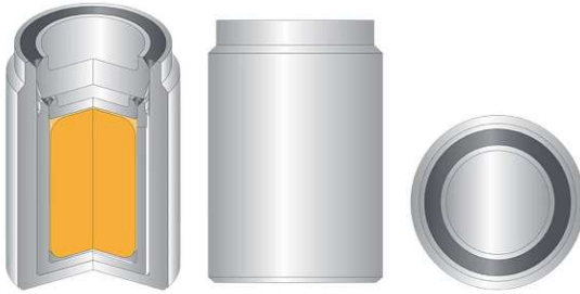
Figure 6.9 Cs-137 sealed source [36].
