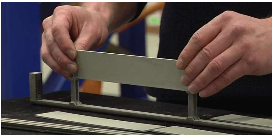
Figure 1.2. Plates of enriched Uranium-235 covered by aluminium alloy that serve as a target to produce Molybdenum-99. [19]
