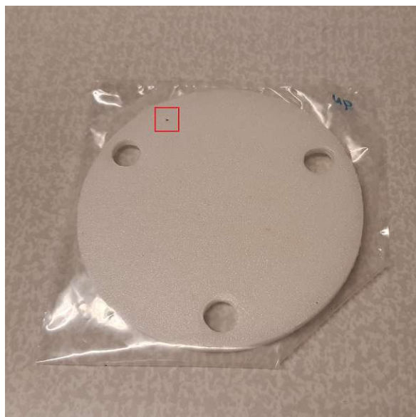
(a) Photo of the passive sampler disk with the particle inside the AIP hotspot region highlighted in red.
