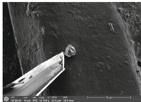
(b) Extraction needle next to the particle (near ion image).
