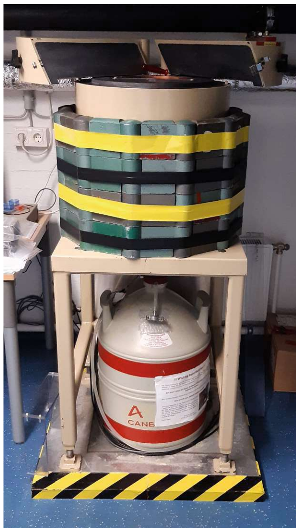
(a) Photo of the low-level gamma spectrometry setup used extensively at the ATI for this thesis. The top shielding consists of the original factory shielding for this setup with an additional layer of lead bricks around that. The nitrogen dewar sits below the detector platform.
