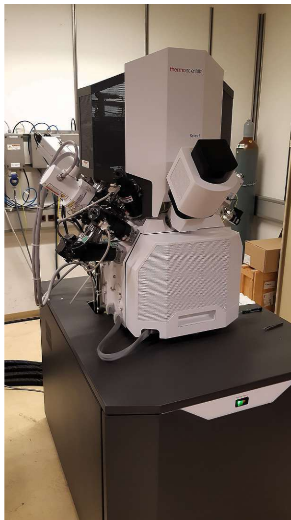
(b) Photo of the Scios 2 DualBeam FIB SEM setup used at the USTEM to do micro-surgery on the samples to extract potential hot particle candidates.
