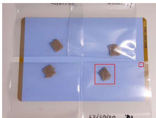
(a) Photo of the quartered corner piece during the very first fractionation cycle. The main sample and the tiny, detached fiber bundle are highlighted in red.
