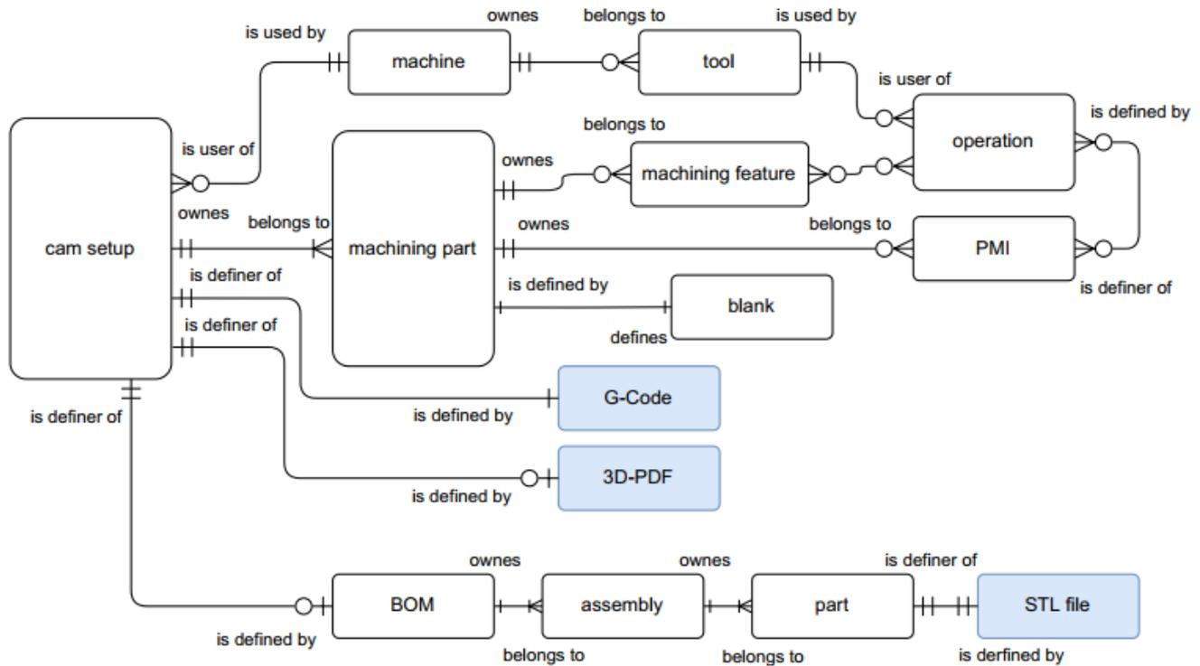
Fig. 2. Illustration of the data entities including relations and relation types in an Entity-Relationship diagram. The blue fields are entities that are stored in their specific document types. This includes STL files, the G-code, and the 3D-PDF. the storage directory must be used to point at these documents.
