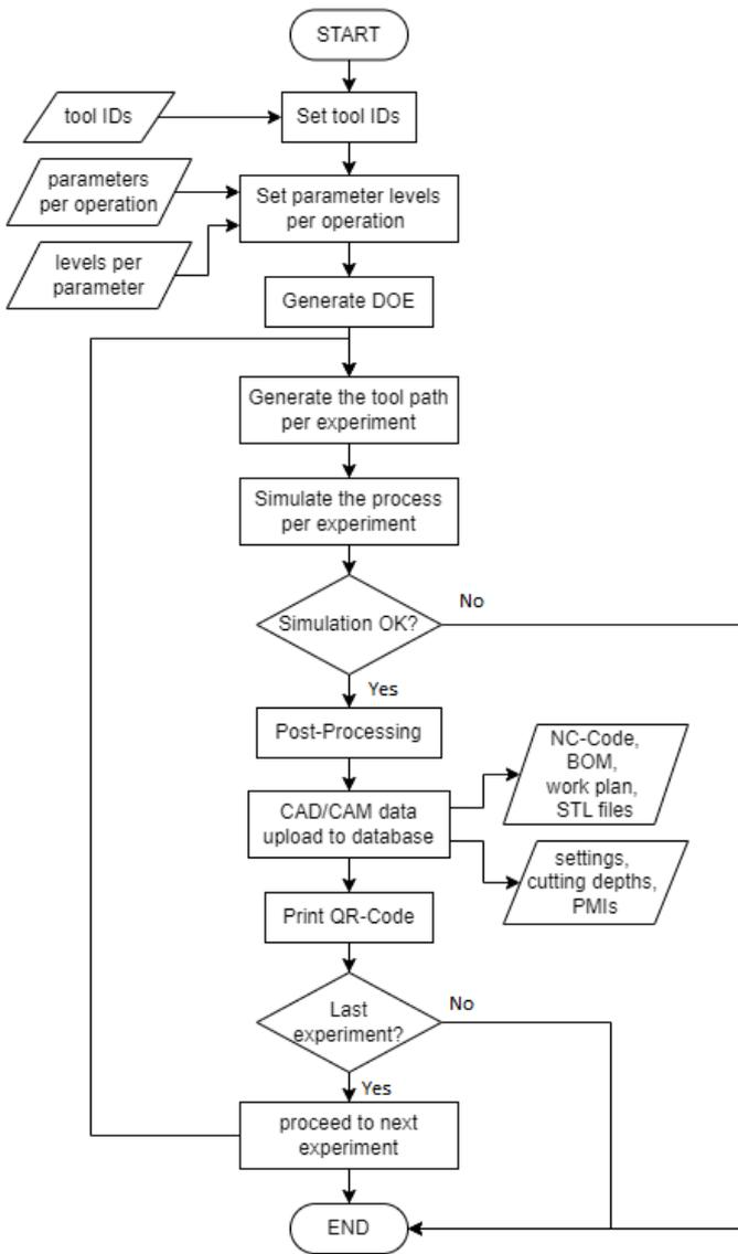
Fig. 3. The flow within the DOE extension for commercial CAM software includes user input for the DOE’s factor level specification. For later tool wear estimations, the function “set tool IDs” waits for the user to state if any tool was changed to allow tool wear estimations. “Print QR-Code” calculates a unique ID before printing a label to put on the blank.
