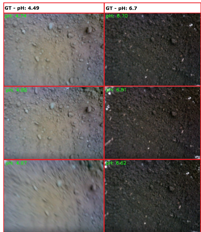
Fig. 8. EDGESOIL 2.0 Performance of pH Prediction on Terrain. EDGESOIL 2.0 performs soil pH prediction on the black and red types of soil on the terrain conditions. On the top left of each frame is shown the predicted pH value, which is compared to the GT value on the top.
