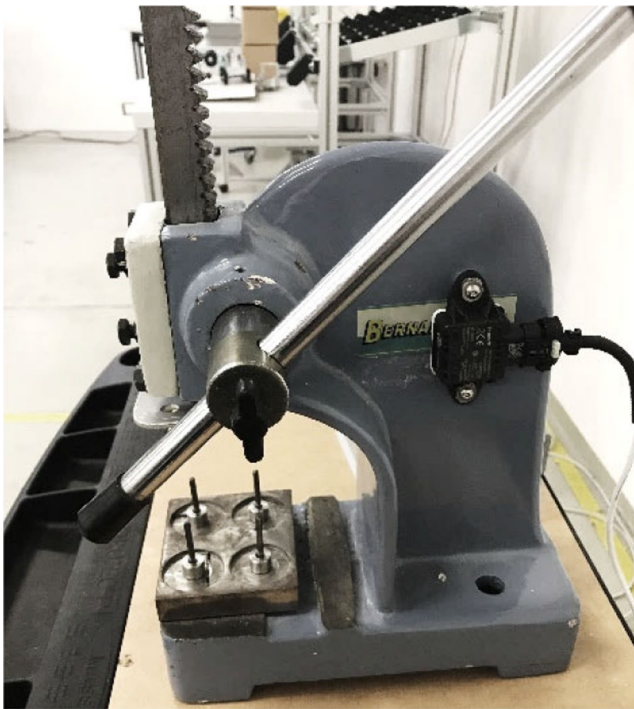
Fig. 8 CISS sensor attached to a manual press
