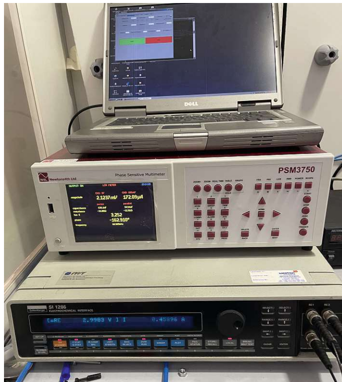
Figure 3.6.: Solartron linked to the PSM3750 and Computer for analysis
