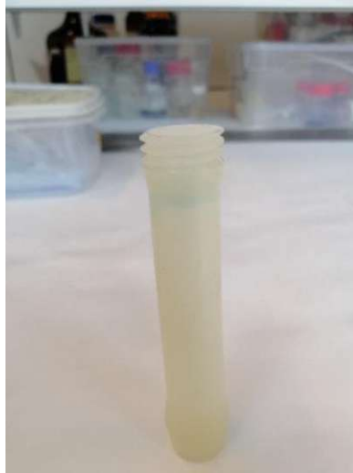
Figure 2 Irradiation capsule used to hold vial with gold foil in liquid during irradiation.
