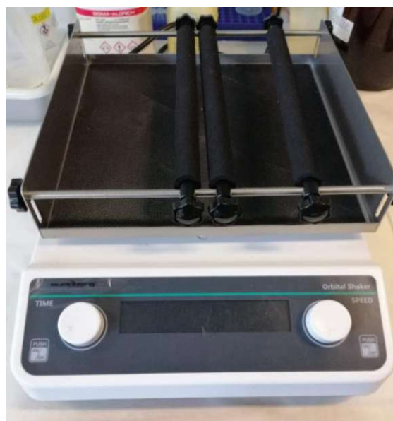
Figure 3 Shaking table used to shake gold foil in liquid via rotation of vial.
