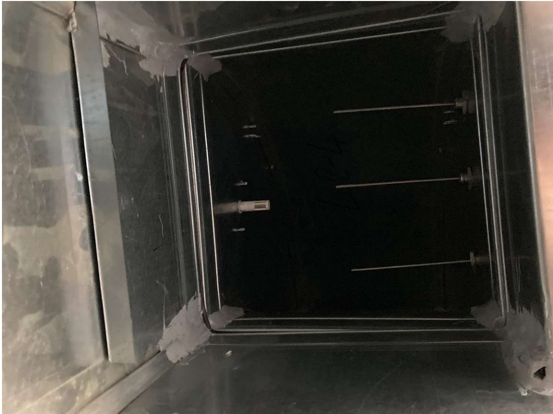
Figure 19: The inside of the air duct with a humidity sensor on the left and three temperature sensors on the right.
