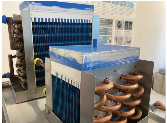
(a) Explosion rendering of the regenerator. (b) The regenerator in the front with the absorber in the back.
