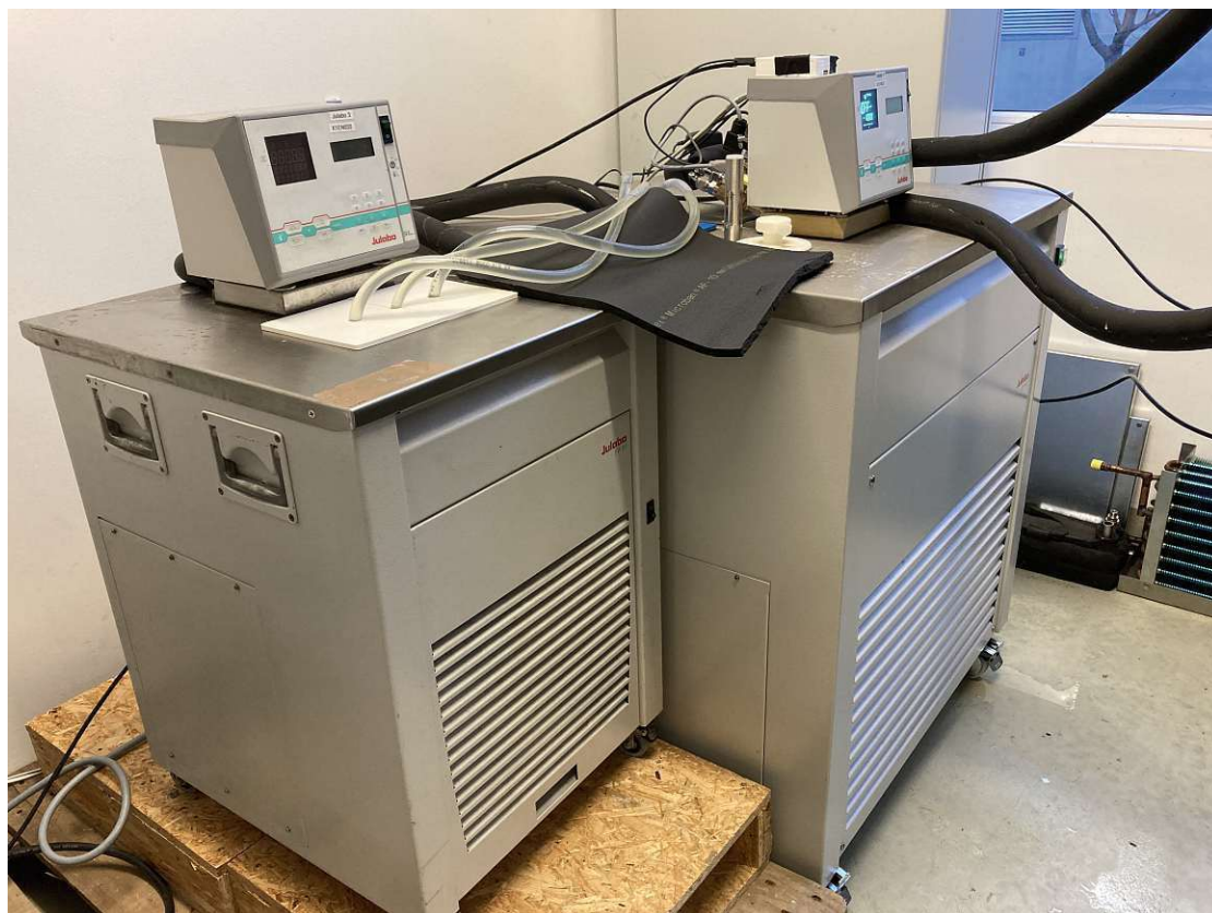
Figure 15: The main Julabo FP55-SL bath thermostat on the right was supported by the smaller Julabo FP51-SL on the left. The internal coolant heights are being leveled by the three connection hoses.
