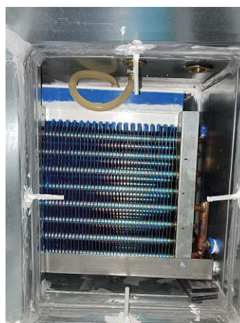
(b) The absorber backside as seen from inside the air duct: The four plastic tubes connect to a differential pressure sensor to measure the pressure drop over the absorber.
