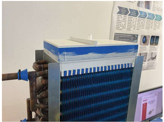
(a) Explosion rendering of the absorber and all 3D-printed parts. (b) Front of the fully assembled absorber.
