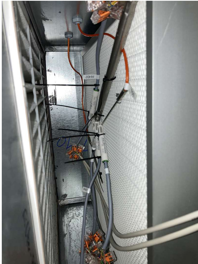
Figure 20: In order to calibrate the humidity sensors, they were mounted on the HEPA-filter using zip ties. The larger one in the middle provides the reference for calibration.
