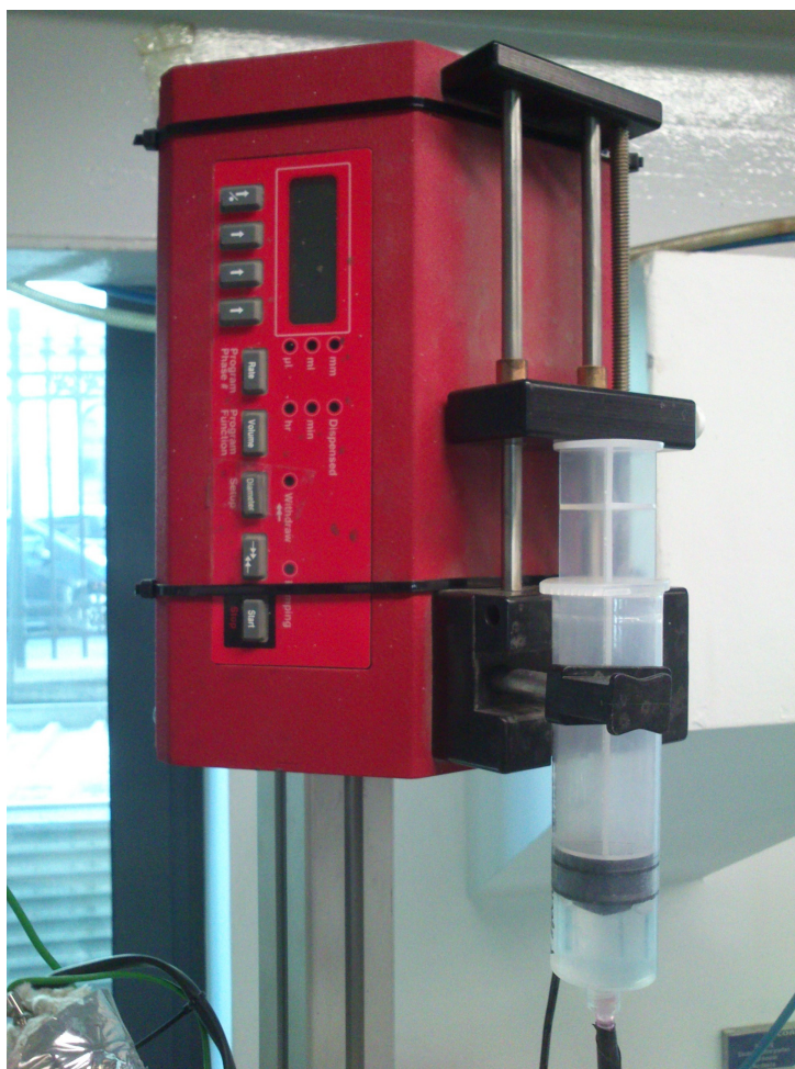
Figure 13: Syringe pump for toluene injection
