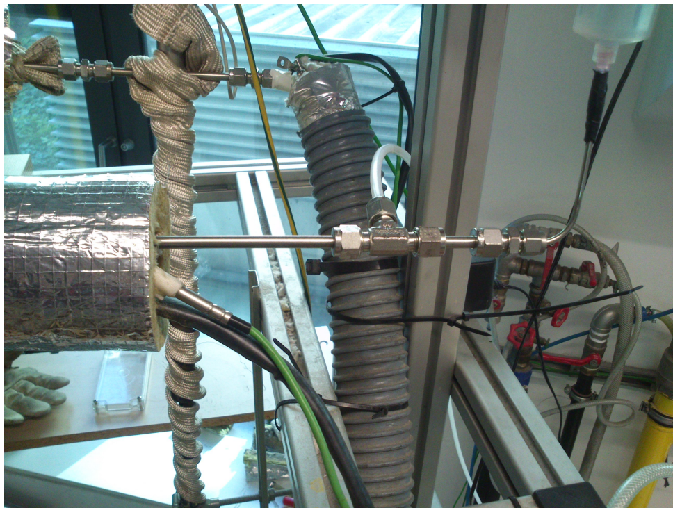
Figure 14: Tee-connector to mix nitrogen with toluene
