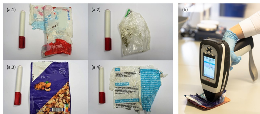
Figure 2. Examples of samples from different fractions used in the experiments: (a.1) PE-PP (PO), (a.2) PE-PA (NPO), (a.3) PET-PE (NPO), (a.4) PET-PP (NPO), and (b) an example of performing measurements with the microPHAZIR handheld spectrometer with copper as measuring background.
