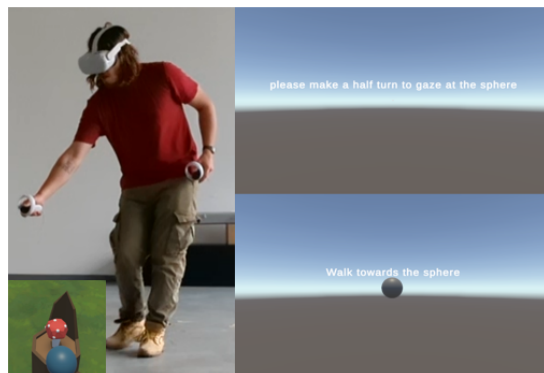
Figure 1: Left - Participants could freely choose between three locomotion techniques (walking, steering, teleportation) during the navigation task. Right - User's view when using the 2:1 Turn technique: top - the user is requested to perform a half-turn rotation to gaze at a sphere; bottom - once the gaze is aligned with the sphere, we ask the user to walk towards to reset the view of the VE.
