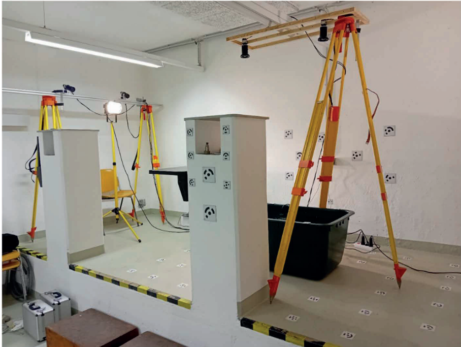
Figure 1: Setup of the lab experiment. Water and stone filled 200L bucket, coded targets serving as control and check points, synchronized camera rig consisting of 2 oblique cameras (left) and 2 nadir looking cameras (top)
