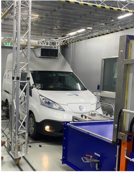
FIGURE 6. Experimental testbed with refrigerator truck. The air temperature at the measurement testbed can be regulated to remain constant at \vartheta_{\text{amb}} = -5^\circ\text{C} , 23^\circ\text{C} and 30^\circ\text{C} .
