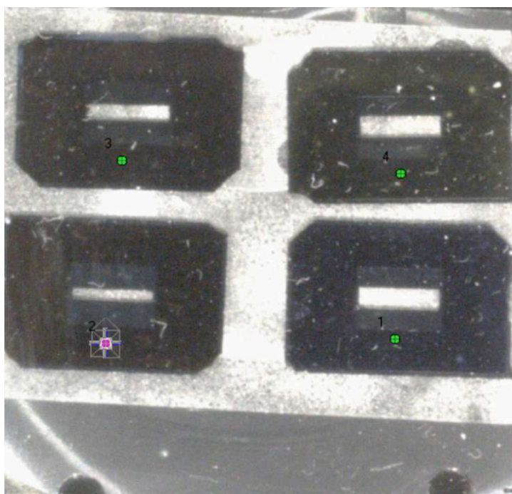
Figure B.2: Chips' regions for the XPS characterization of the Si/N content ratio.
