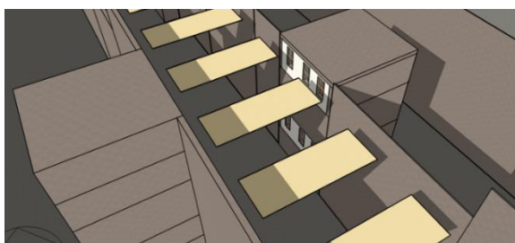
Fig. 12. Simulation model for indoor thermal conditions (18m high shading elements, 15 th April 03:00 pm; Illustration: The Authors)
