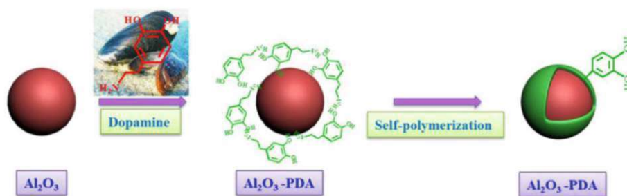
Figure 2.14 Schematic diagram of polydopamine functionalization by dopamine polymerization on top of on \text{Al}_2\text{O}_3 nanoparticles 120 .
