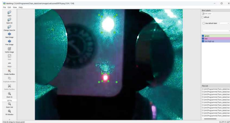
Figure 6.3: A screenshot of the software labelling.[27] The rectangles indicate the location of an object and the colour indicates the class. The detected classes are also listed in the column on the right side of the picture.
