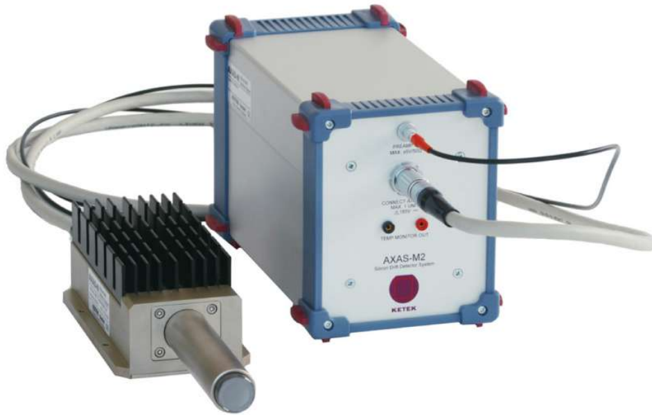
Figure 4.2: The detector including the detector electronics [23]
