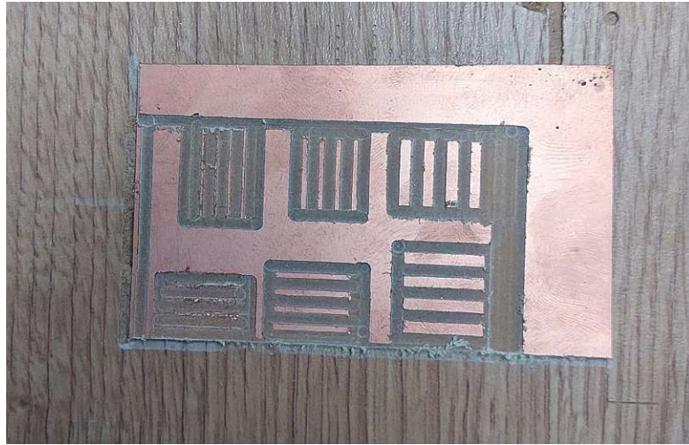
Figure 8.12: A picture of the pattern milled in the epoxy board.
