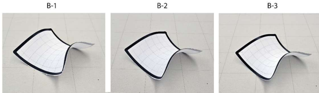
Figure 55: resulting tiles - uniform pre-stretching (25%) and uniform boundary cross sections
