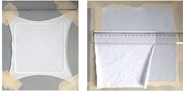
Figure 26: manual pre-stretching with tape used for clamping
