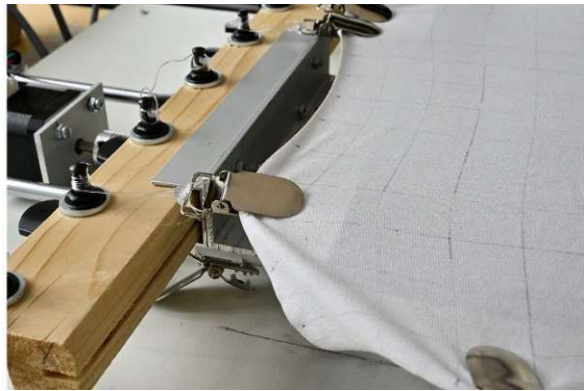
Figure 36: left: pointwise clamping mechanism with individual pins, right: linear clamping mechanism
