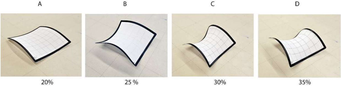
Figure 45: resulting tiles with increasing amounts of stretching.
