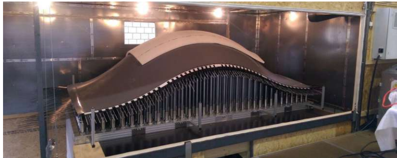
Figure 13: fabrication principle of ADAPA mold (Raun & Kirkegaard, 2015)
