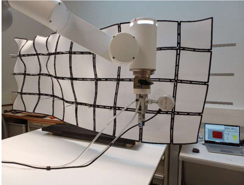
Figure 73: scanning procedure with Intel RealSense L515 LiDAR camera and the aid of a 6-axis collaborative robot
