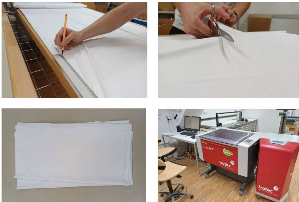
Figure 112: fabrication steps of individual tiles – textile preparation
