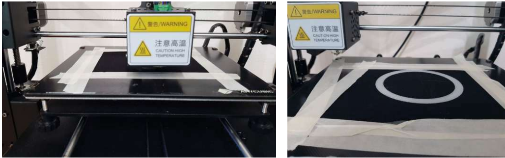
Figure 28: using a FDM 3D printer with a pre-stretched piece of fabric fixed to the print bed
