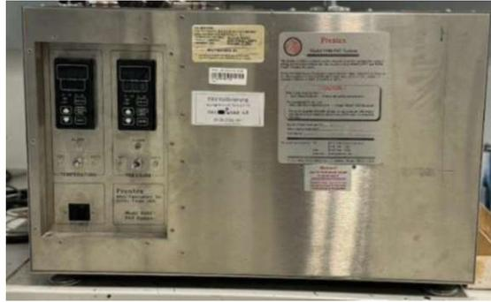
Figure 13: PAV Vessel in the laboratory
