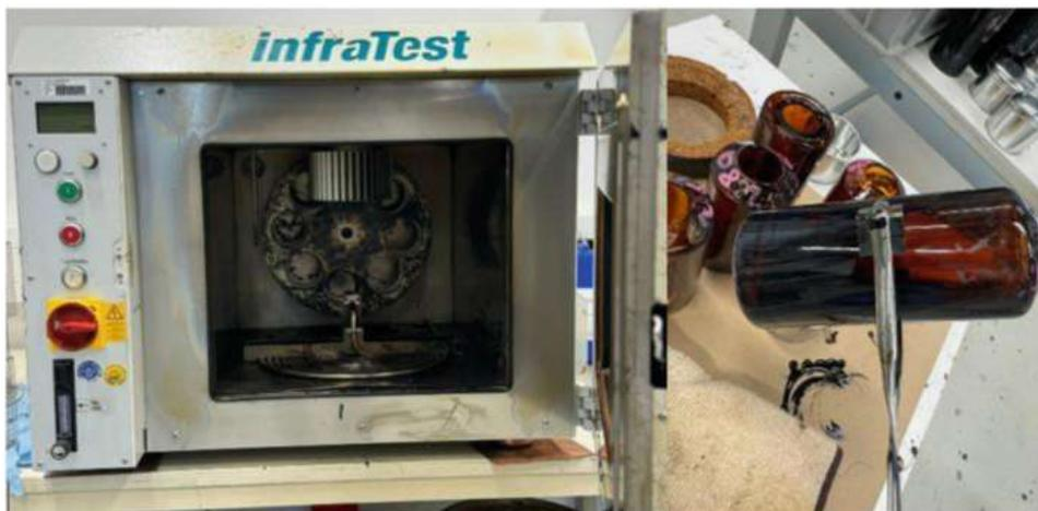
Figure 9: Rolling Thin Film Oven(left) and Binder after the RTFOT (right)
