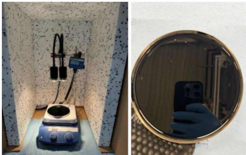
Figure 18: LA3 25W and 50 W lamp and Binder 1 after 3 days of light ageing
