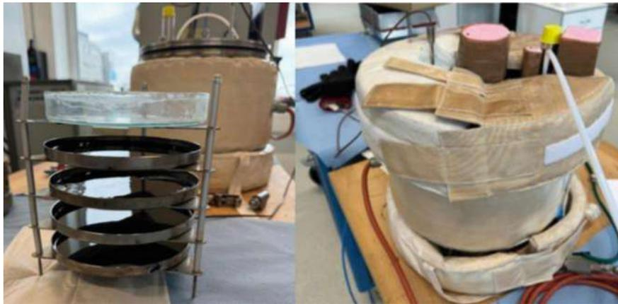
Figure 14: VBA stack of 4 aluminum trays (left) VBA vessel (right)
