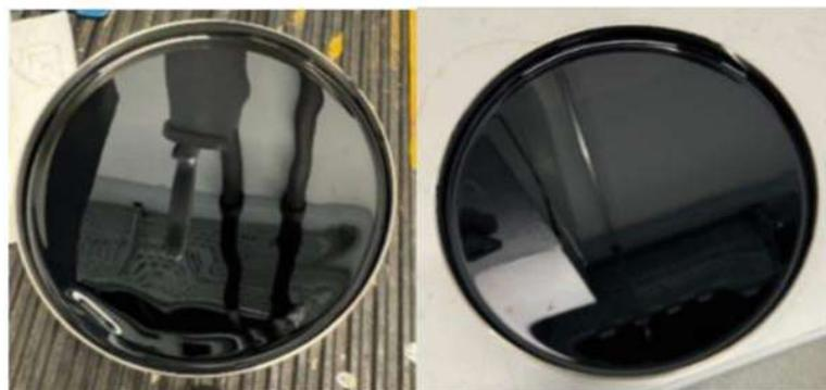
Figure 12: Bio-binder 1 short-term aged after PreVBA (left), bio-binder 2 short-term aged after PreVBA (right)
