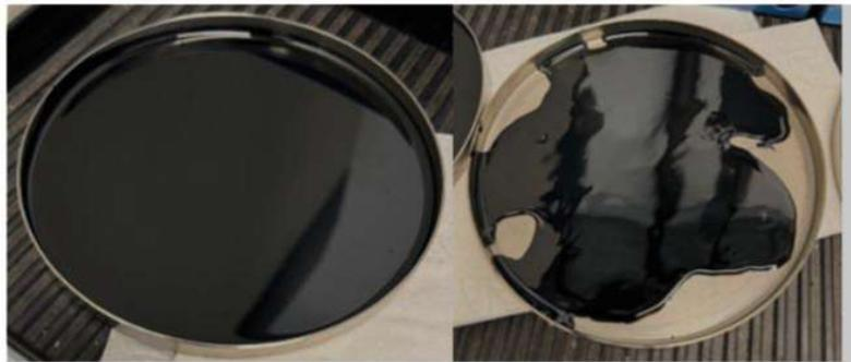
Figure 11: Binder 1 short aged after PreVBA, binder 2 short aged after PreVBA
