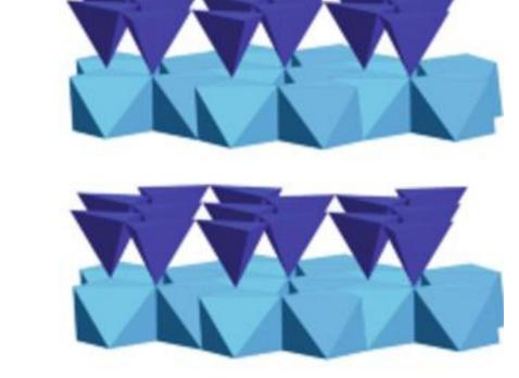
Kaolinite 1:1 layer T-O Silica Tetrahedral layer (T) Alumina octahedral layer (O) No interlayer ions
