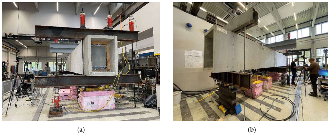
Figure 6. Test setup and measuring equipment: (a) View of the load application area (Section A–A). Hydraulic presses in red, including loading cells. (b) View of Sections B–B and C–C. Transducers placed on yellow wooden panels to measure the deflection of the webs.
