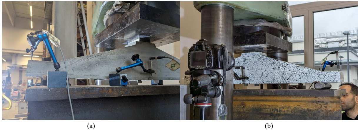
Figure 2. Test setup and monitoring concept: (a) LVDTs at support and midspan and (b) stochastic pattern for DIC observation
