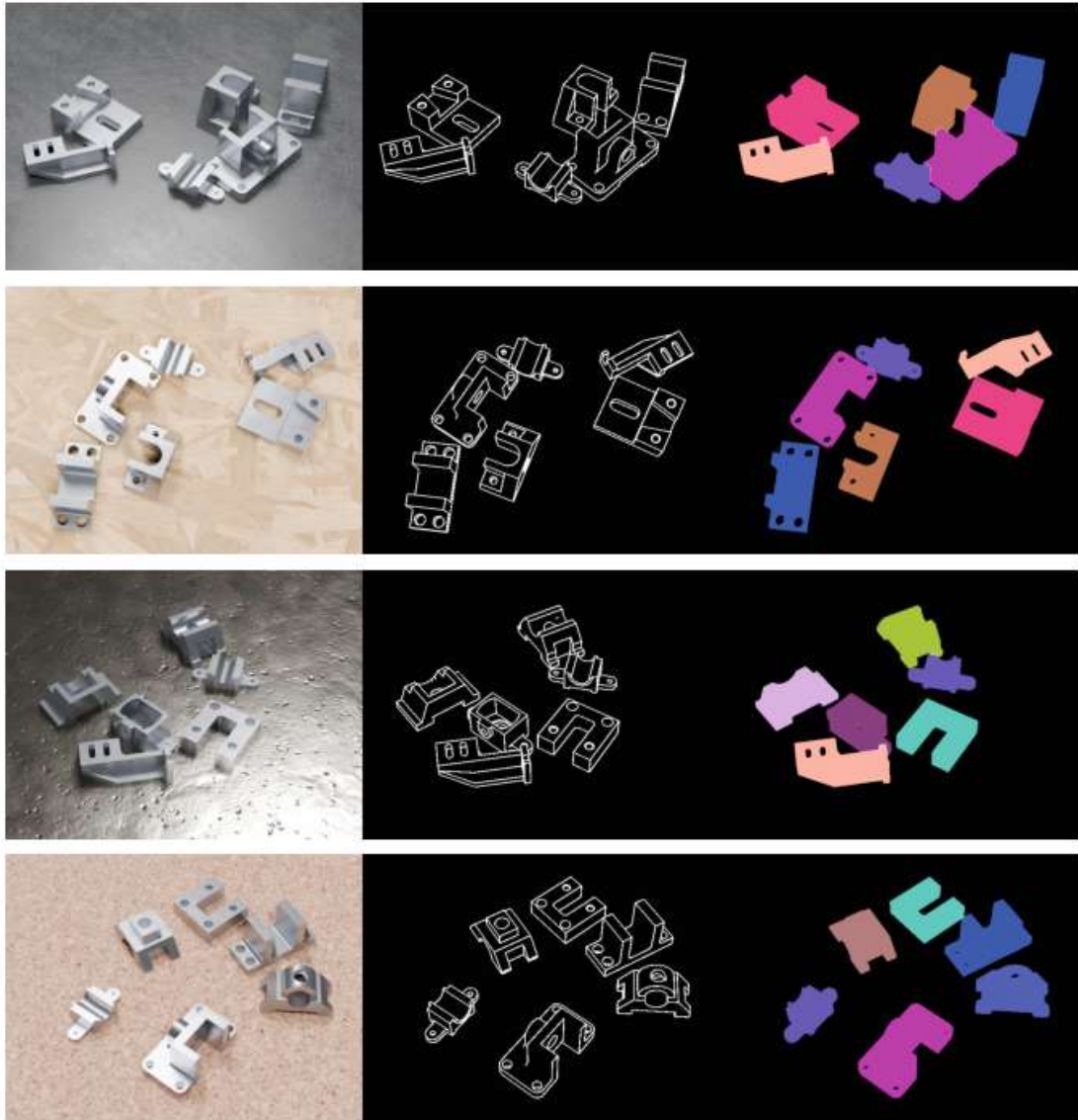
Figure 3.6: Samples of synthetic training data with RT-Less [10] models. From left to right, the RGB scene image, edge images, and segmentation masks. The individual masks are color-coded for improved clarity.
