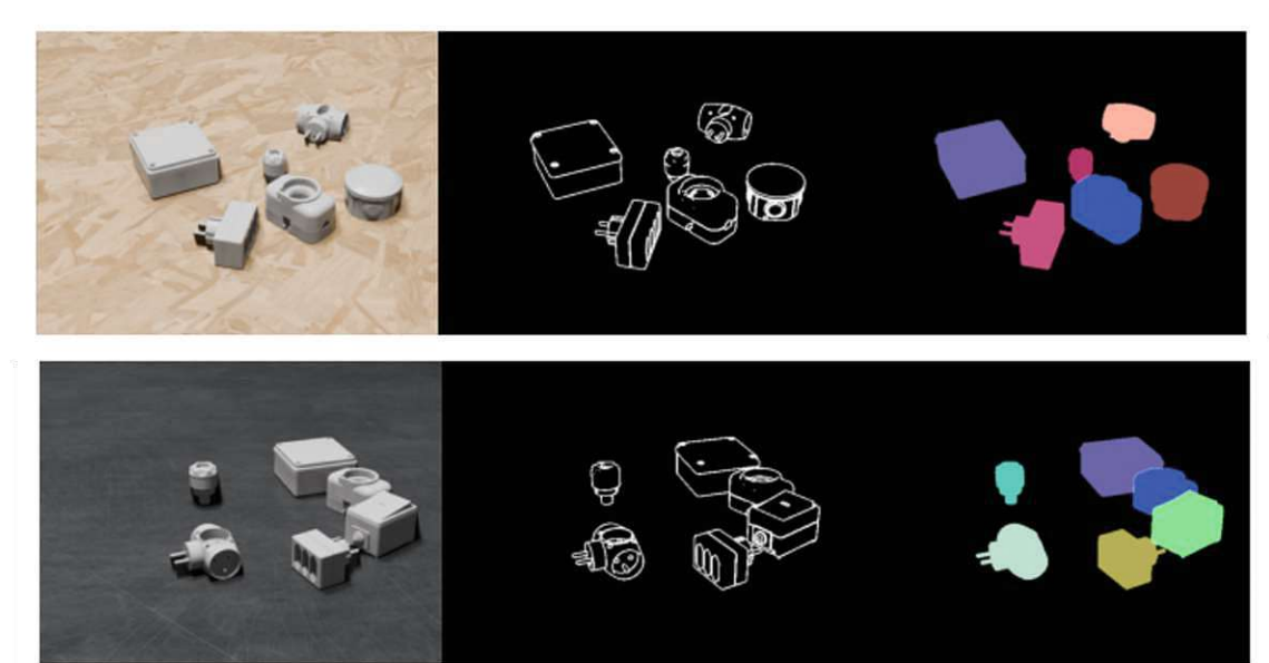
Figure 4.12: Samples of synthetic training data with T-Less [32] models. From left to right, the RGB scene image, edge images, and segmentation masks. The individual masks are color-coded for improved clarity.
