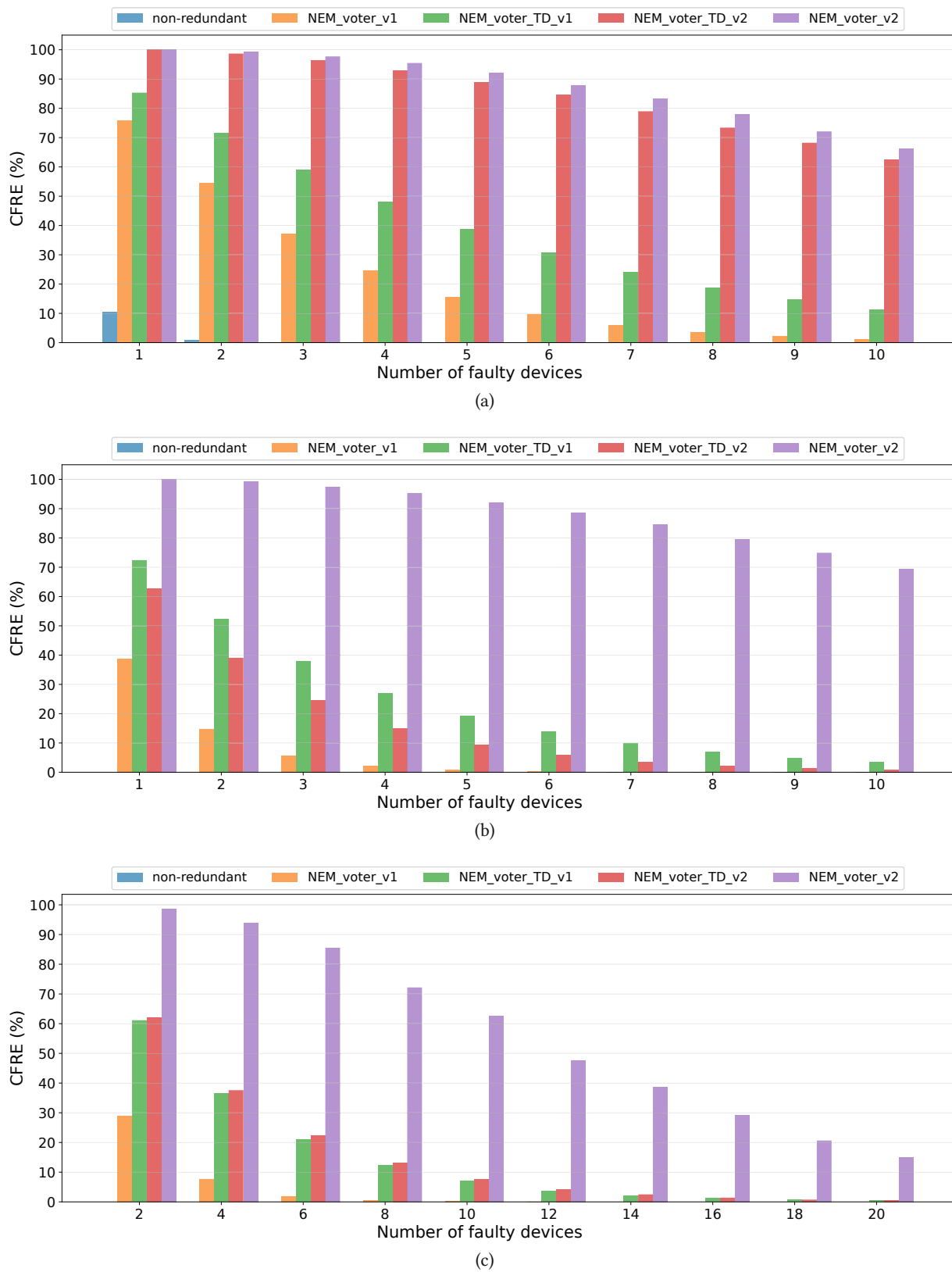
Figure 6.11: CFRE for the full adder with TMR applied at gate level and NEM voter designs: (a) stuck-off, (b) stuck-on, (c) mixed faults (50%/50%).
