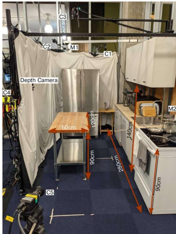
Figure 3.4: Placement of the environmental cameras in the recording space. M1-2 denote the microphones, and C1-5 the cameras. Records of the depth camera were not published. Source: [1]
